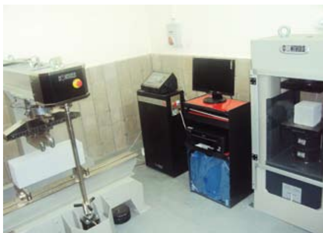
Compression Test Apparatus with Controls
