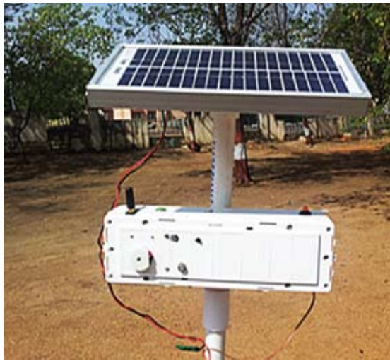
Solar Powered Air Pollution Monitoring System Based on IITH-Mote
