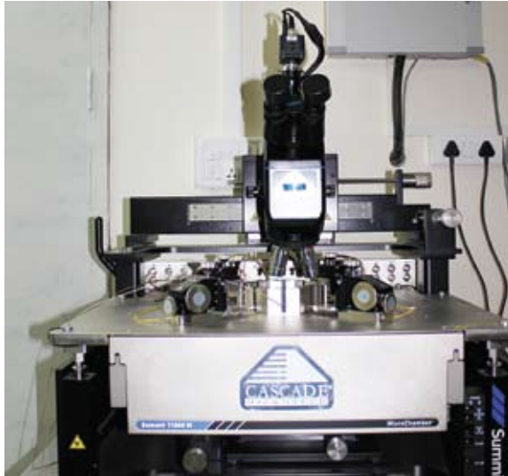
Electrical characterization system with probe
